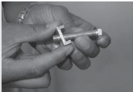
Fig 5.1.2 M10 x 60 screw to be fixed with U-profile in the installation rail.
