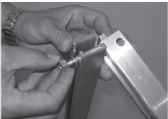
Fig 5.1.3 Attach with washer and nut to vertical installation rail. (Insert until end of long whole)
