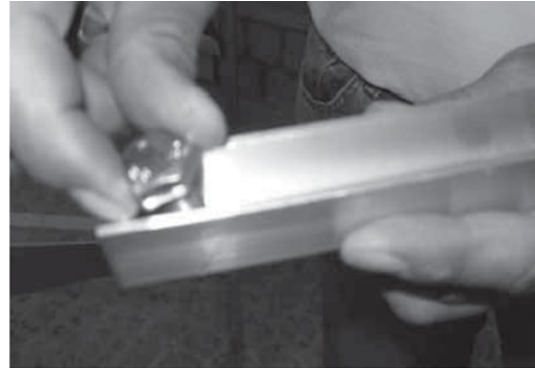
Fig 5.1.20 Both M12 x 20 screws have to be inserted in the connection rails for the upper and below horizontal rail as shown.
