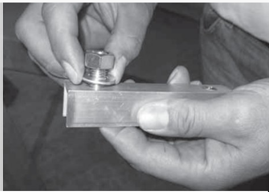
Fig 4.2.16 On the opposite side the u-washer and nut have to be inserted and have to be tightened easily by hand.
