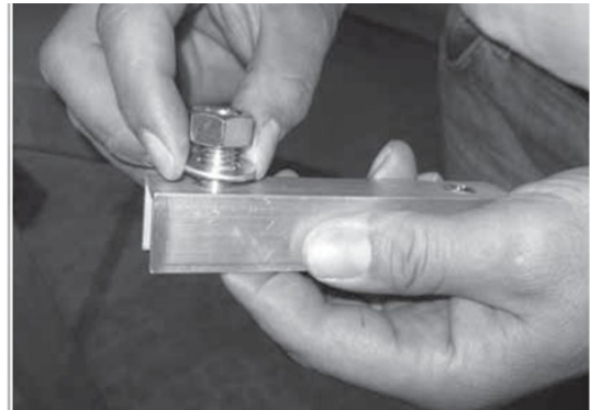
Fig 5.1.21 On the opposite side the u-washer and nut have to be inserted and have to be tightened easily by hand.
