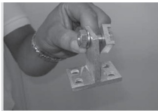
Fig 5.1.6 M10 x 30 screw to be inserted in the U-profile and through the boring above in the T-piece. It is softly fixed with washer and nut.
