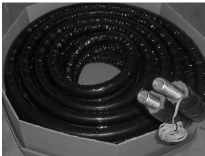
Fig 6.0.1 Roth 2 in 1 Flexible quick-installation pipe made of stainless steel, pressure resistant. Solar system supply and return line in a high temperature resistant insulation sleeve. 49' (15m) to a box.
