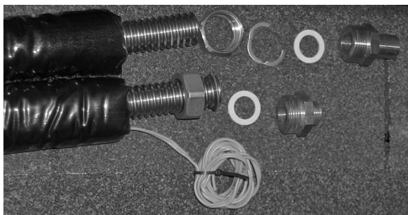
Fig 6.0.3 The pipe can easily be cut using a standard tube cutter. Once the proper length has been determined an cut. The connections are made with oval clip collar set. The nut is slipped over the pipe and the oval clip is pressed over the pipe to form the assembly.
