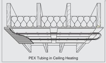
Some building codes require that the pipes be pressurized while the concrete is poured. PEX tubing is made for rough handling at a building site, so it can be virtually ignored (walked on, etc.) during the pour. 1/2" PEX tubing is flexible, installs quickly and easily, and the installed cost is a fraction of its value as a lifelong insurance towards future energy crises and the resale value of the building.
