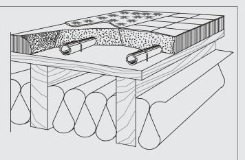
PEX Tubing in Gypsum Overpour on top of suspended floor
