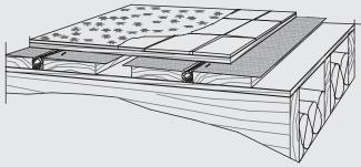
PEX Tubing with Alu Panels over suspended floor
