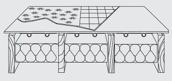
PEX Tubing installed from underneath in suspended floor
