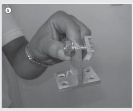
**5.** M10 x 30 screw to be inserted in the U-profile and through the boring above in the T-piece. It is softly fixed with washer and nut.
