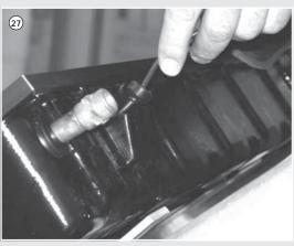
27. Remove the cable lead at the return of the collector field and slide it over the cable of the temperature sensor: temperature insert sensor into the immersion sleeve as far as possible and remount the cable lead in the collector.
