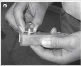
**20.** On the opposite side the u-washer and nut have to be inserted and have to be tightened easily by hand.
