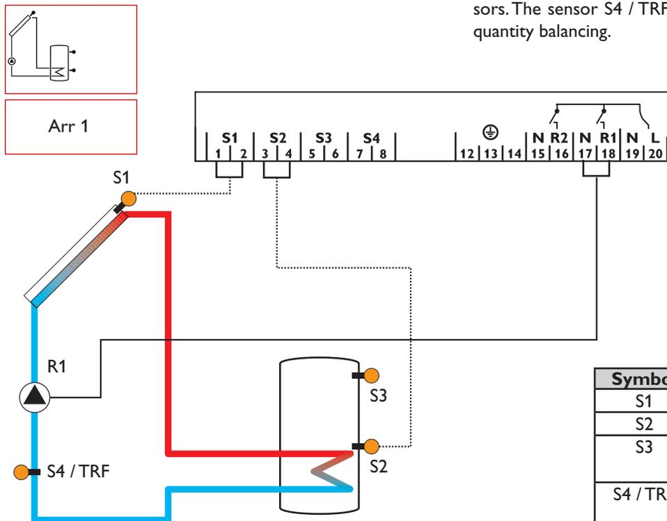
**Standard solar system** with 1 tank, 1 pump and 3 sensors. The sensor S4 / TRF can optionally be used for heat quantity balancing.
