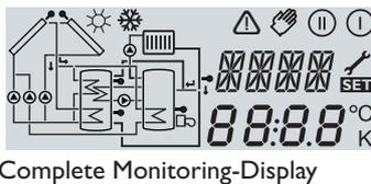
The system monitoring display consists of 3 blocks: **indication of the channel, tool bar and system screen** (active system scheme).
