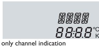
The **indication channel** consists of two lines. The upper line is an alphanumeric 16-segment indication in which mainly the channel names / menu items are shown. In the lower 7-segment indication, the channel values and the adjustment parameters are indicated. Temperatures and temperature differences are indicated in °F / °C or Ra / K.
