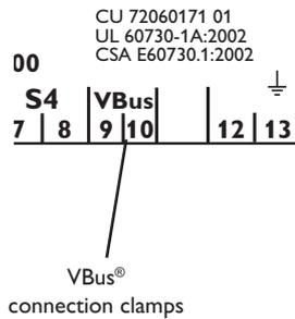
The controller comes with aVBus® for data communication and energy supply of external modules. The connection is effected with optional polarity at the clamps marked with „VBus®“. Via this data Bus you can install one or more VBus® modules, e.g.:
