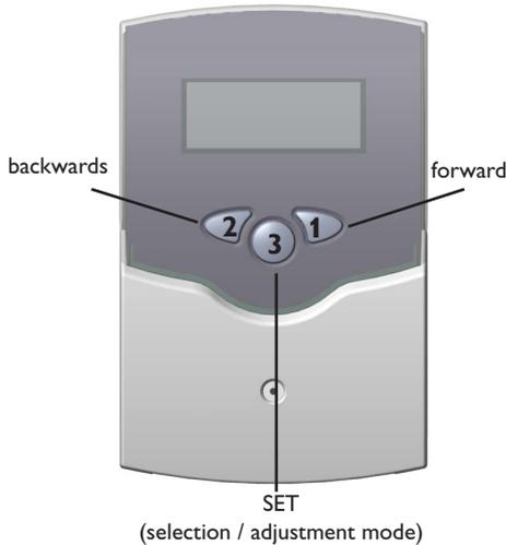
The controller is operated by 3 pushbuttons below the display. The forward-key (1) is used for scrolling forward through the indication menu or to increase the adjustment values. The backwards-key (2) is accordingly used for the reverse function.
