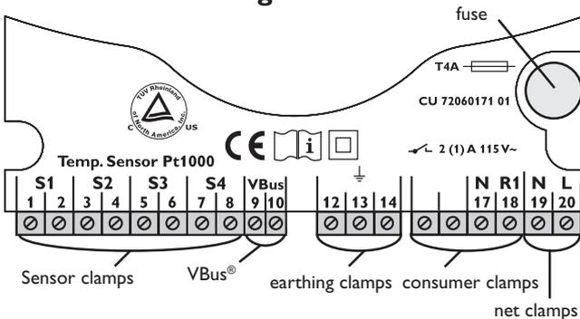
The power supply to the controller must only be made by an external power supply switch (last step of installation!) and the line voltage must be 115 Volt (50...60 Hz). Flexible lines are to be fixed at the housing by enclosed strain relief supports and screws.
