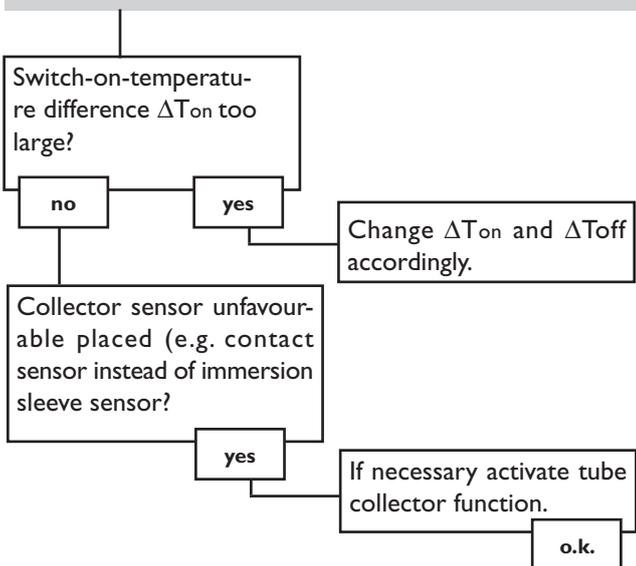
The temperature difference between tank and collector increases enormously during operation; the collector circuit cannot dissipate the heat.
